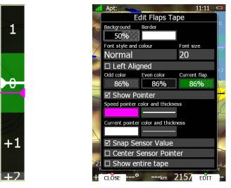
Magenta pointer shows required flap settings. White pointer shows selected flap position. Selected flap position band is coloured with green colour, when matching flaps are set. When wrong flaps are set, then selected flap band will be coloured red.
