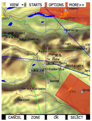
Move cross to task point to pick it and move it around. Move cross to task leg to insert point.
