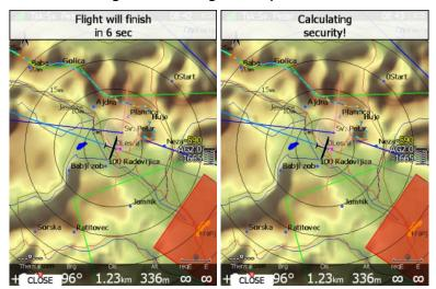
The flight is finished when the message Calculating security disappears. At that moment the statistics page will be changed back to logbook view. Now it is safe to switch off the instrument.
