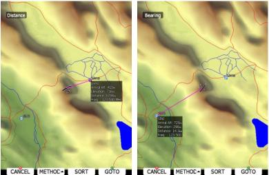
Details of selected airport will be drawn next to it. In upper-left corner of screen current sort method is shown. There are two possibilities, distance sort or bearing sort. Press SORT button to change it.
