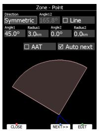
Using parameters in the zone dialogue it is possible to describe all types of observation zones. **Angle12** defines the orientation of the observation zone. Available values for **Direction** are:
