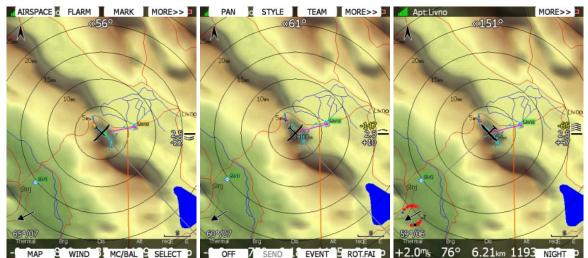
Press the **MORE>>** button to see more options. If the remote stick is available the behaviour is slightly different. When the check button is pressed on the remote stick a menu will appear instead of the button functions.
