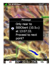
A message will appear. If you confirm this with **YES** the task will be advanced to the next turn point and it will recalculate the task taking the optimal fix as the task point.
