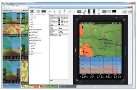
If new profile is created with LX Styler, it will have default device settings. However, it is possible to copy device settings from profile to another profile. Select newly created profile as active profile. Select profile from which you would like to copy settings to active profile. Press **COPY** button. A confirmation dialog will open.
