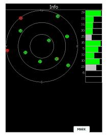
Green satellites are satellites currently being used for position determination. Three concentric circles represent satellite elevation (0, 30, 60 degrees above horizon). If a satellite is in the centre of the circles it is directly overhead.
