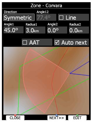
Using parameters in the zone dialogue it is possible to describe all types of observation zones. **Angle12** defines the orientation of the observation zone. Available parameters for **Direction** are:
