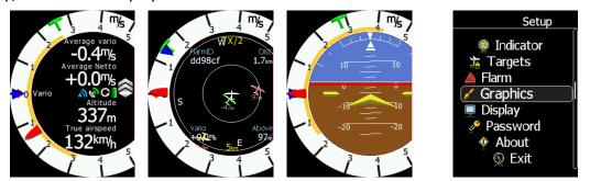
Press middle button for long time to enter setup menu. In setup menu it is possible to setup graphic interface for Flarm radar screen and numeric values. Numeric screen can also be setup on main display unit.
