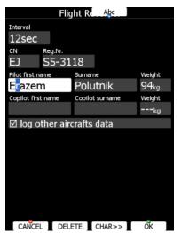
Press the **CHAR>>** button to advance the cursor to the next position. The cursor can also be moved to next position using the bottom-left knob. Rotate it clockwise to move forward. **The Abc** button is a toggle button and will change the letter case. Press it to toggle modes.
