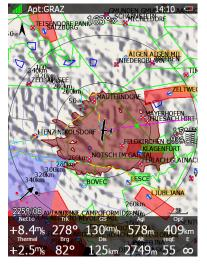
Use **Show glider range area** to display reachable area from current altitude with current wind and MacCready settings. Use **area colour** and **area border** to define its properties. Press the **DEFAULT** button to reset these settings back to default.
