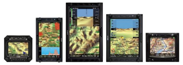
Extremely bright colour display readable in all sunlight conditions with backlight automatically adapted using an ambient light sensor (ALS).
