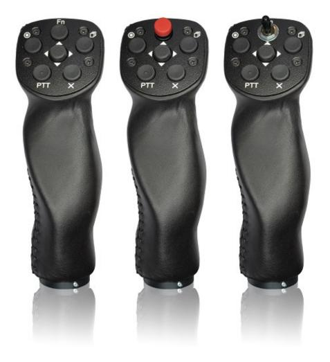
The stick is available also in various diameters: 18 mm, 19.3 mm, 20.3 mm, 24.4 mm and 25.4 mm. All necessary electronics is built into the top of the stick. The four coloured wires from the bottom must be connected to RS485 splitter. Additionally two shielded cables are used for speed to fly command and push to talk button.
