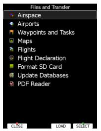
Within a profile user can selected different airport databases, airspace and waypoint files. Selected files can be stored inside main display unit or on inserted SD card or USB stick. It is also possible to upload files from SD card or USB stick to main display unit.
