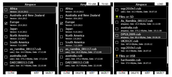
Select the required airspace and press **SELECT**. If a check mark is shown in front of an airspace item, this airspace file will be shown in the graphics and used for proximity calculation, when enabled.
