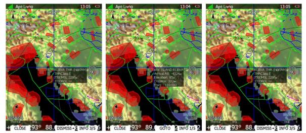
A blue cross will be plotted over the screen with info box for given cross position. Move cross up and down on map using PAGE selector knob. Move cross left and right using MODE selector knob. Turn ZOOM selector knob to zoom map.
