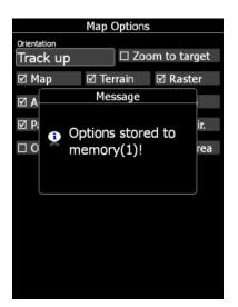
Press button **MEM 1** for a long time. A message "*Options stored to memory (1)*" will be displayed and the settings are stored. Change the settings a little bit. Press button **MEM 2** for long time. A message "*Options stored to memory (2)*" will be displayed and the settings are stored to memory location 2. Now short pressing of **MEM 1** will invoke the saved settings from memory 1.
