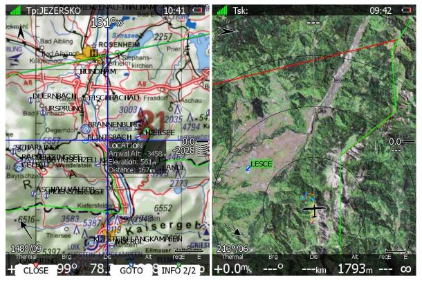
The system is supporting two file formats: CMR file format provided by SeeYou software from Naviter. There are available free of charge sectional maps of USA (<u>www.soaringdata.info</u>) and QMP file format provided by Ifos. Please contact Ifos (<u>www.ifos.de</u>) or (<u>www.strepla.de</u>) to purchase scanned maps.
