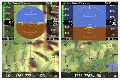
Shape of symbol can be customized as well. You can also enable to display sky directions with checking "Show compass" property.
