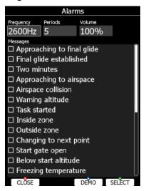
**Frequency** and **Periods** define the length and pitch of alarm. Press **DEMO** button to play alarm sound. Change volume to define loudness of alarm.
