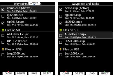
Multiple files can be selected. All checked files will be shown on the graphics page and used in the near mode calculation, if the waypoint is of the proper type (airport or outlanding place). However, only one file can be the active file. The active file is primary used for task creation.
