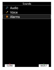
Volume can be also controlled using upper left rotary knob. Rotating it will directly change volume for sounds, which is currently being played. For example, if voice message is being played, voice message volume will be set. If alarm is beeping, alarm volume will be set. In speed to fly mode, speed to fly volume is set and in climb mode, vario volume is set.
