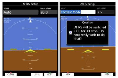
Place you glider in levelled position and press LEVEL button. You can also modify pitch offset, if you rotate PAGE selector knob. More detailed can be pitch set using pitch offset spin control.
