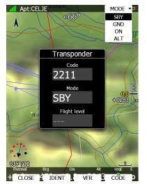
Use **MODE** to select mode of operation of connected transponder. Press **CODE** to enter squawk code. Press VFR to automatically set squawk code to 7000. Press **IDENT** to identify.
