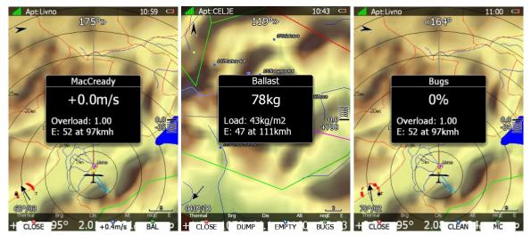
Use the PAGE selector knob to modify the MacCready setting. In the middle button there is a suggestion for the MacCready setting which is based on the last four thermals. Additionally to the selected MacCready value an wing loading is also shown together with the calculated glide ratio with corresponding speed.
