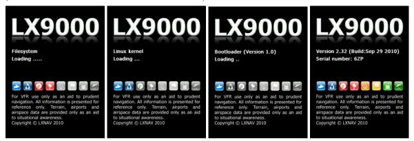
The boot procedure normally takes up to 20 seconds but in the case of a firmware update or system check it can take more time. The final boot screen displays information about the LX90xx system firmware and the IGC serial number. When the boot procedure is completed the profile selection dialogue is shown. Please refer to Chapter 8.1 for more details about starting up the system.
