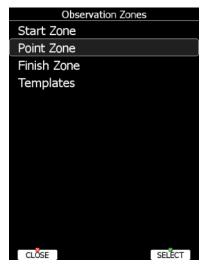
Each type of observation zone is defined with two angles, two radii and mean bearing (**Angle12**). These parameters enable the creation of any known zone geometry separately for start, turn point and finish.
