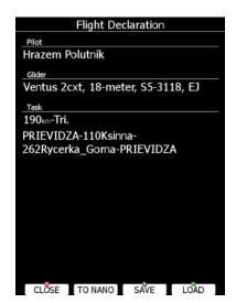
On the screen pilot, glider and task information are shown. Press the **SAVE** button to save the declaration onto a SD card or USB stick. Press the **LOAD** button for loading. If Nano flight recorder is connected to USB port, **TO NANO** button will appear. Press it to transfer declaration to Nano flight recorder.
