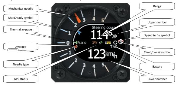
**Mechanical needle** displays vario, netto, relative or speed to fly value. It can be setup separately for climb mode or cruising mode. Printed scale can be chosen in range from -5 to 5 or from -10 to 10. Within software range can be set to 2.5, 5, 10m/s or 5, 10, 20kts or 500, 1000, 2000fpm.
