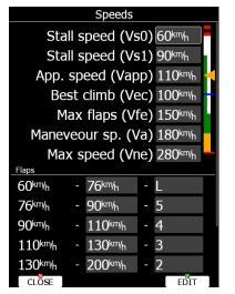
Once speed range is entered, the system will be able to display requested flap position based on current wing loading and g-factor.
