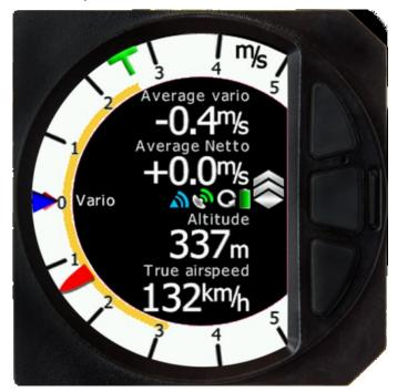
Indicator basic screen is split into two parts, white ring with needle and vario scale. Additionally to needle, blue MacCready triangle, green thermal average T and red diamond for 20 seconds average are shown. In the middle four user-customizable numbers are shown. When middle button on indicator is pressed display will toggle between numeric display, Flarm radar display and artificial horizon screen.
