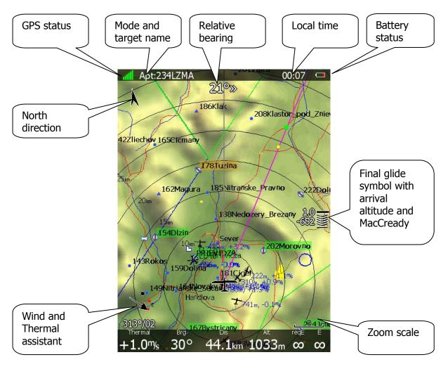
In the top row the GPS status is shown. Green colour represents GPS 3D, yellow colour means GPS 2D and red colour is GPS bad. The number of coloured bars indicates the number of visible satellites. Each bar represents two satellites.
