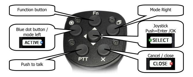
Remote stick has six push buttons and on multi-directional button in the middle. Move multidirectional button left and right to zoom in and out. Move it in up and down direction to select different page of to move on menu. Press it to select and item or to invoke a menu in navigational mode.
