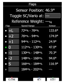
When all flap positions are set, a green dot will be displayed with current flap position. If flap labels are not set yet, press EDIT button to name flap label. Flap labels must me entered with increasing speed range. It is recommended that flaps labels are set together with speed range in Polar and Glider setup. See Chapter 5.1.13 for more details.
