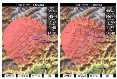
In the upper-right corner the remaining task distance is shown as well as the required task speed, remaining task time, delta time and estimated time of arrival.
