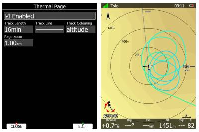
Previous navigational page will be restored when your aircraft will stop circling. You can also manually exit thermal mode by rotating PAGE or ZOOM knobs.
