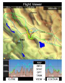
A map with flown path is shown and barogram. Use **ZOOM** selector knob to zoom in or zoom out flight. Use PAGE selector knob to move through flight. Press **VIEW** button again to toggle between map view and different statistical pages.
